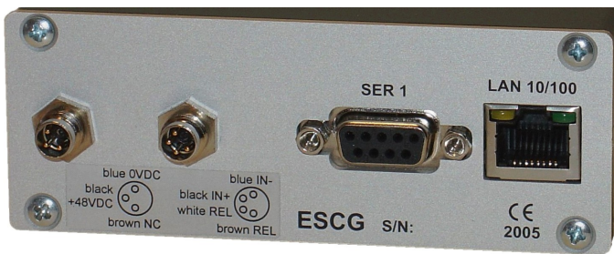
Illustration 24 Rear panel with relay and power connector
